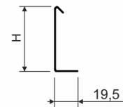
**surface finish:** S - Pre-Galvanized according to EN 10346, EN 10143, zinc-layer 13-27 μm
