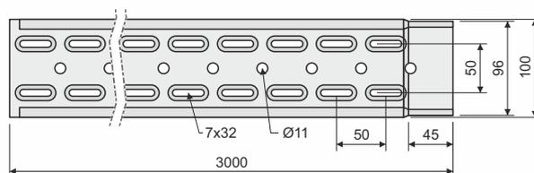
surface finish: S - Pre-Galvanized according to EN 10346, EN 10143, zinc-layer 15-27 µm
