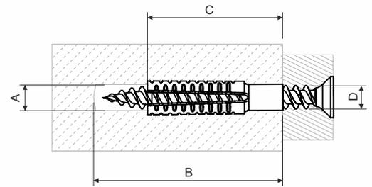
product description: For pre-assembled mounting in concrete, porous concrete, vertically perforated bricks, natural stone with a dense structure, solid brickwork blocks, solid sand- lime bricks.
